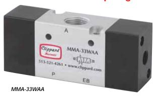
Maximatic® 3-way air piloted valves are either double pilot or single pilot, spring return in #10-32 thread to 1/2" NPT port sizes. These air piloted valves have 1/8" NPT external pilot ports.
