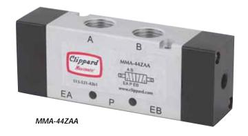
Maximatic® 4-way air piloted valves are either double pilot or single pilot, spring return in #10-32 thread to 1/2" NPT port sizes. These air piloted valves have 1/8" NPT pilot ports.
