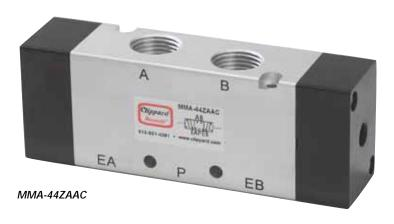
Maximatic® 4-way 3-position double air pilot valves with closed center, pressure center or exhaust center spools are available in #10-32 thread to 1/2" NPT port sizes. These air piloted valves have 1/8" NPT external pilot ports.
