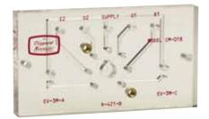
Operation: Supply air passes to port 1 of the R-421 and to supply ports of the ET-3M valves. R-421 is a three position, center closed valve, spring centered. Electronic signal to either ET-3M will pilot R-421 giving corresponding output as long as that ET valve remains energized. Energizing both ET valves simultaneously will cancel out opposing pilots. Springs will return R-421 to center-closed position.
