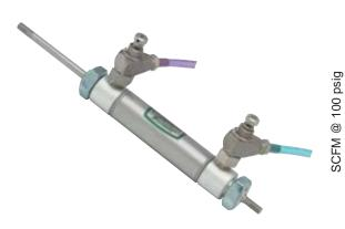
Clippard offers five models of adjustable flow controls with #10-32 through 3/8" NPT ports. They feature a combination needle and check valve that controls flow in one direction and allows free flow in the opposite direction.
