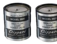
Designed to be piloted by a Clippard EV or ET manifold mount electronic valve. Output from the EV/ET actuates the valve to produce outputs up to 22 SCFM at 100 psig. Combines low wattage, long life and cool running of the EV/ET valves with quick response and high flow of Clippard booster type valves.
