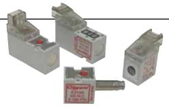
Another feature of the Clippard 10 mm valve is the ability to detach the coil and connector from the valve body. This can be useful for the purpose of orientating the coil by 180°, or exchanging connector types or voltages.
