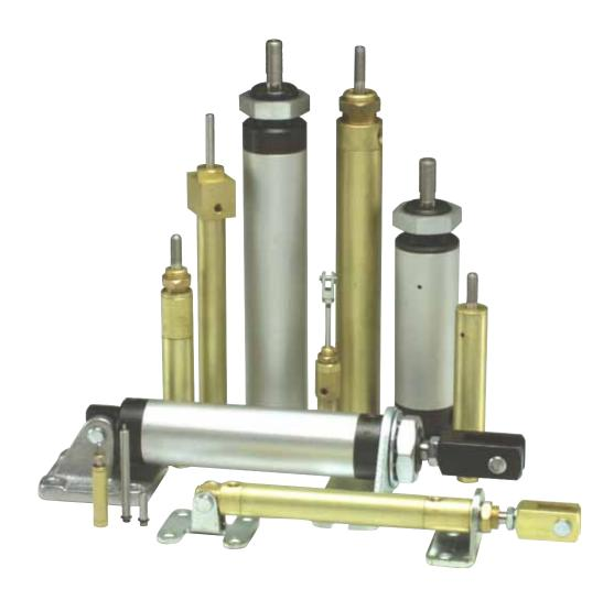
Clippard offers more types of miniature pneumatic cylinders for the designer's convenience, including: spring return, spring extend, air retract, double-acting and double rod models. From sub-miniature (5/32" bore) to heavy duty (1 1/8" bore), the extensive Clippard line provides a wide selection of bore sizes to suit any application requirement. An even wider range of strokes are available in the complete Clippard line of miniature cylinders, in stroke sizes ranging from 1/4" to 20".
