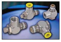
These combination needle and check valve flow controls are typically used to control air flow from air cylinders, thereby controlling the speed at which
